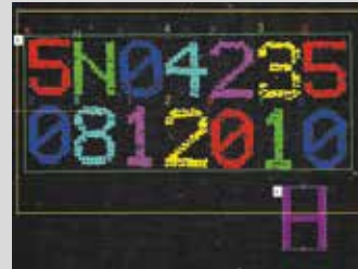
Optical character reading Dot matrix printing can also be read with OCR.
