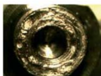
Standard copper paste. Metal pick-up very visible = GALLING
