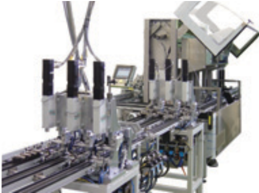
Assembly line equipped with electro-mechanical assembly presses
