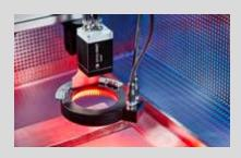
Raised or recessed object details — such as embossed digits and characters on a credit card — are difficult to detect with standard image processing methods. A remedy for this problem was found in the new Multishot function of VISOR® vision sensor range of SensoPart.
