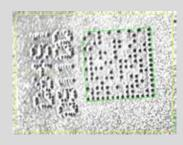
**Dot-peened code on rough substrate** Code is made legible by powerful read-
