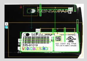
VISOR® Allround — Object detection in color plus identification united in one device. The VISOR® Allround is a real multi-talent among vision sensors. In the allround version, the device combines the functions of the object sensor (i.a. calibration, pattern matching, contour, calliper, BLOB) with the powerful tools of the code reader (barcode, datamatrix and optical character recognition).
