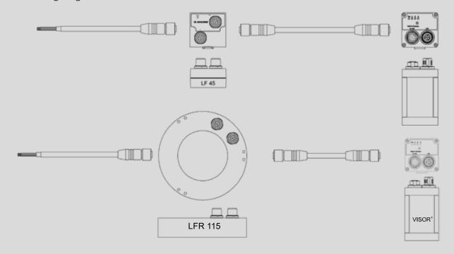
External lighting (panel light LF 45, ring light LFR 115, spot illumination LS) can be connected directly between the vision sensor and power supply.
